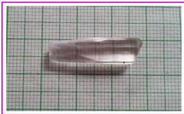
**Figure 3** <110> LS single crystal grown by Unidirectional method
